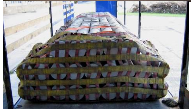
Fastening net and securing of load against movement by front lashing with 4 straps (8 branches) and a net
