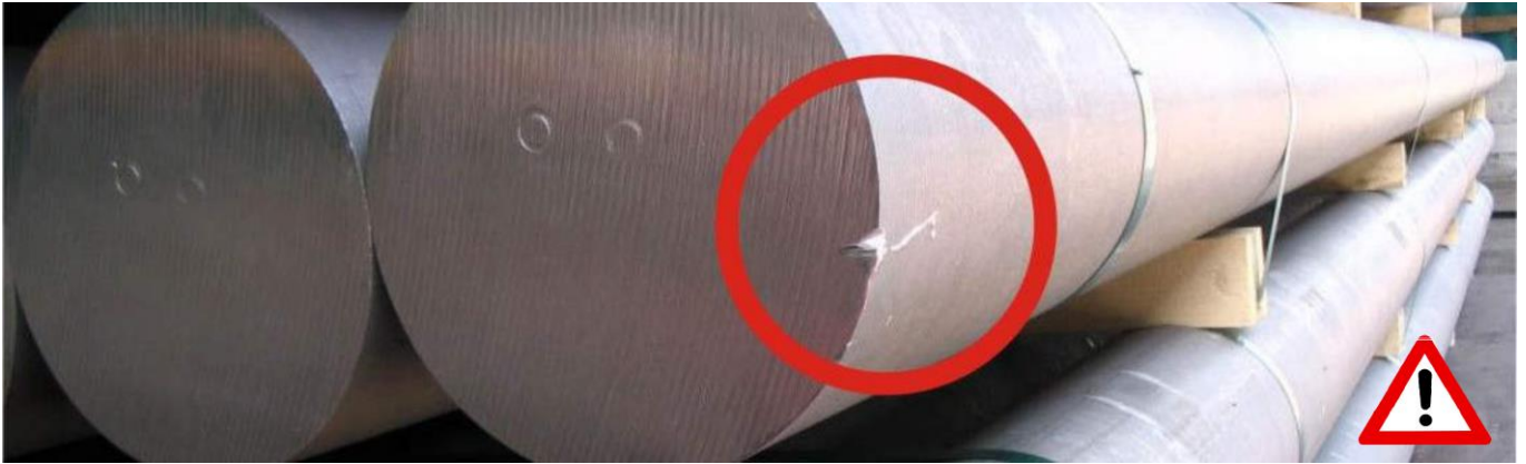
Pressure mark from fixation wall on extrusion ingot!!!
