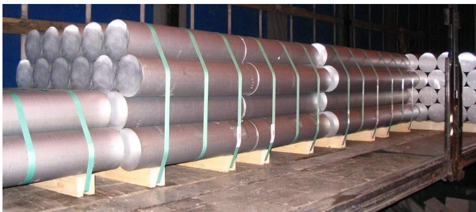
Packages of short extrusion ingots loaded in semitrailer; the compact layout ensures blocking
