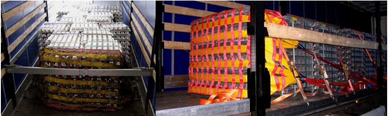
Front fastening of PFA ingots by a net - 4 front double lashings up to 20 tons
