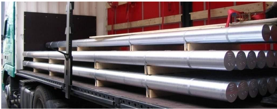
Loading of 6 m extrusion ingots - 2 sections - the first one blocked by the front end wall
