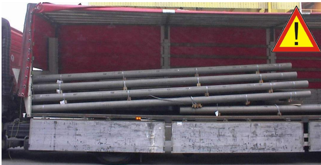
7-meter extrusion ingots moved forward during braking and broke/crashed in the semitrailer front end wall
