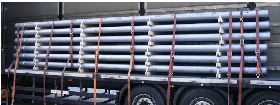
Nakládka čapov - dĺžka 7 m - 1 section in the middle of the semitrailer - 6 layers
