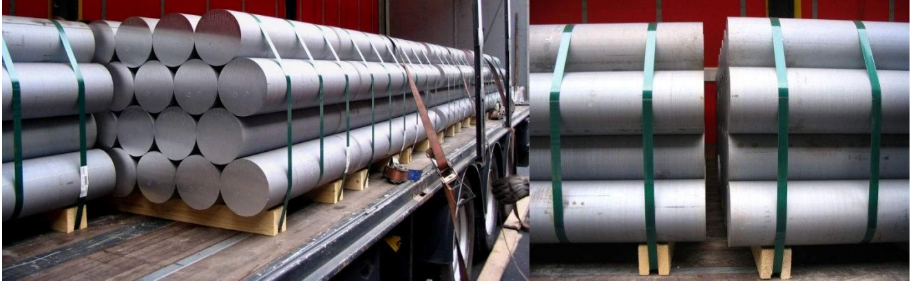
Placement of short extrusion ingots and the gap between the packages - minimize the gaps!
