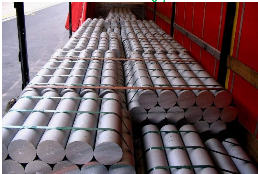
Placement of short extrusion ingots and the gap between the packages - minimize the gaps!
