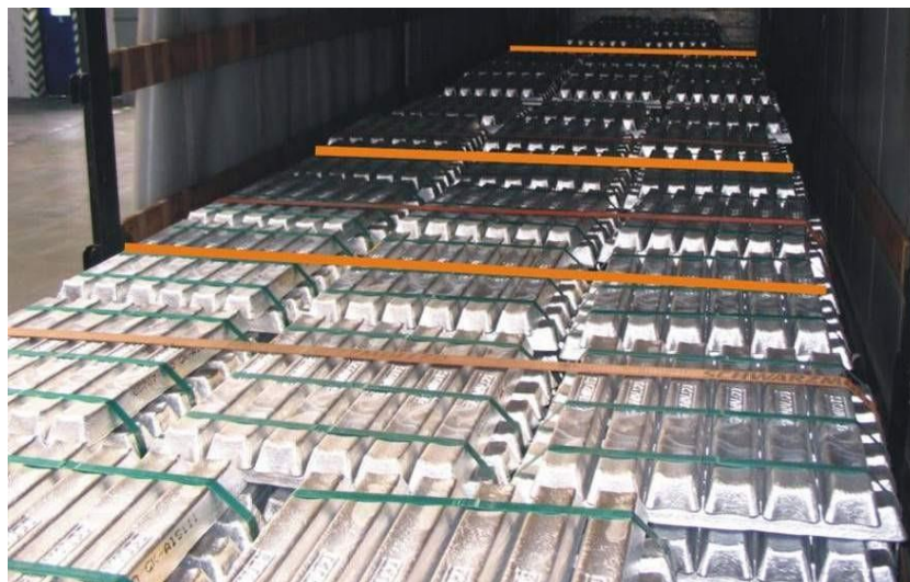
PFA ingots placed in a compact way (42 units) - each section fastened by top lashing - cargo blocked against sufficiently strong front end wall
