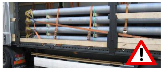
Incorrectly fastened net; the strap is secured only in two fastening points!!!
