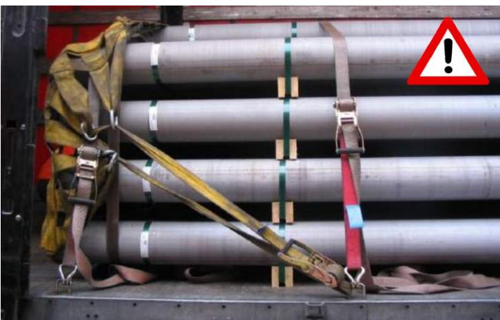
Incorrectly fastened net; the strap is secured only in one fastening point with the strength of 2000 daN!!!
