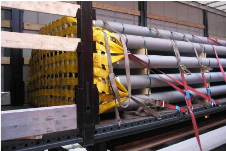
Securing of cargo by front lashing with 4 straps (8 branches) and a net - sufficient fastening
